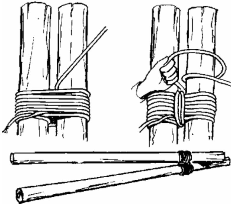
1. Lay out the poles. For most lashings you will want to lay the poles side by side with the butt ends aligned (thicker ends).
