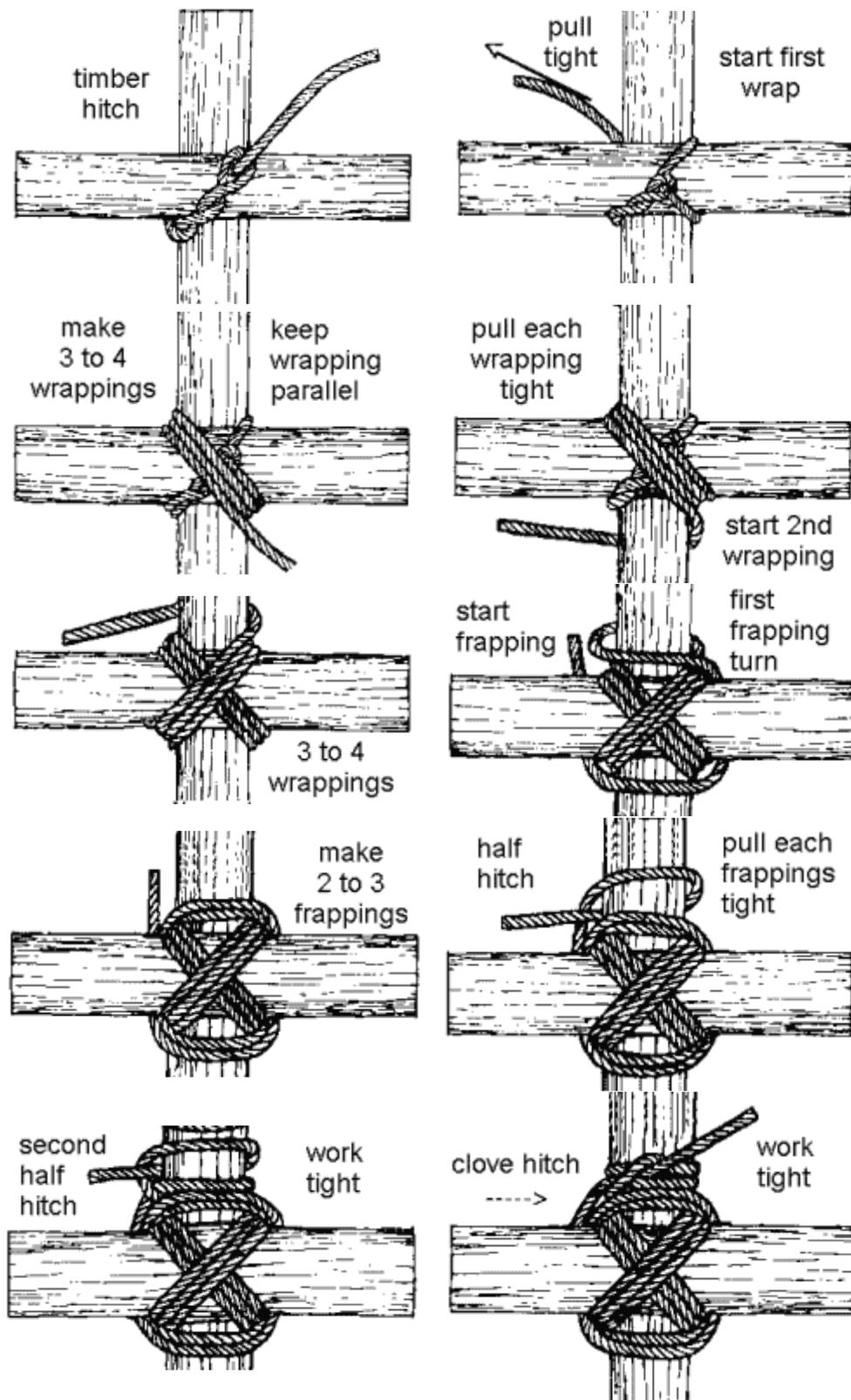
1. Tie a timber hitch diagonally around both poles.
