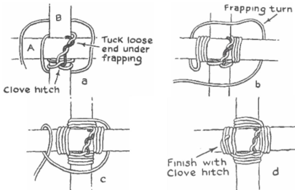
1. Start by crossing the two sticks or dowels at perpendicular or 90 degree angles.
